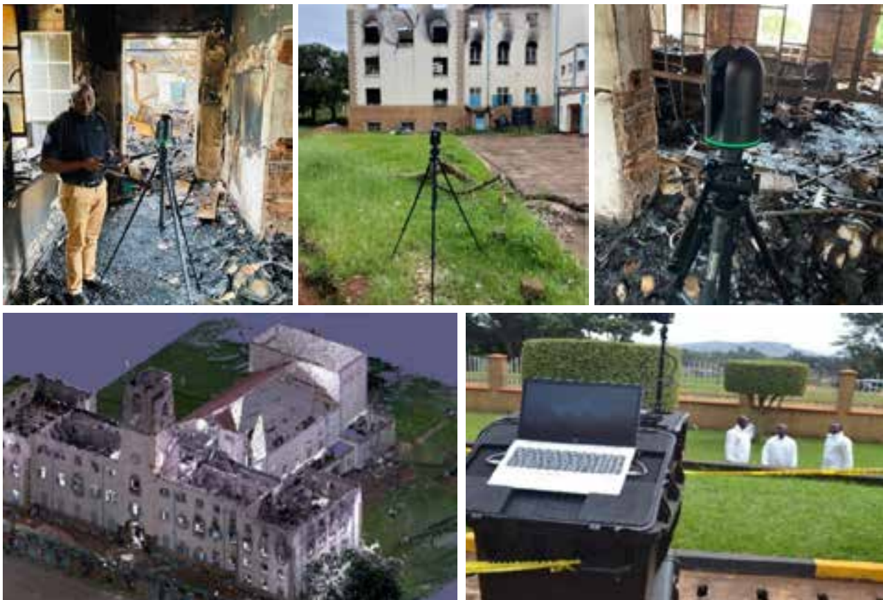
Figure 24: Showing one of the 3D Crime Scene Photogrammetry equipment in use.
